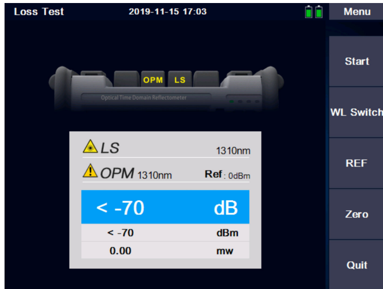
Light Source Module Interface
